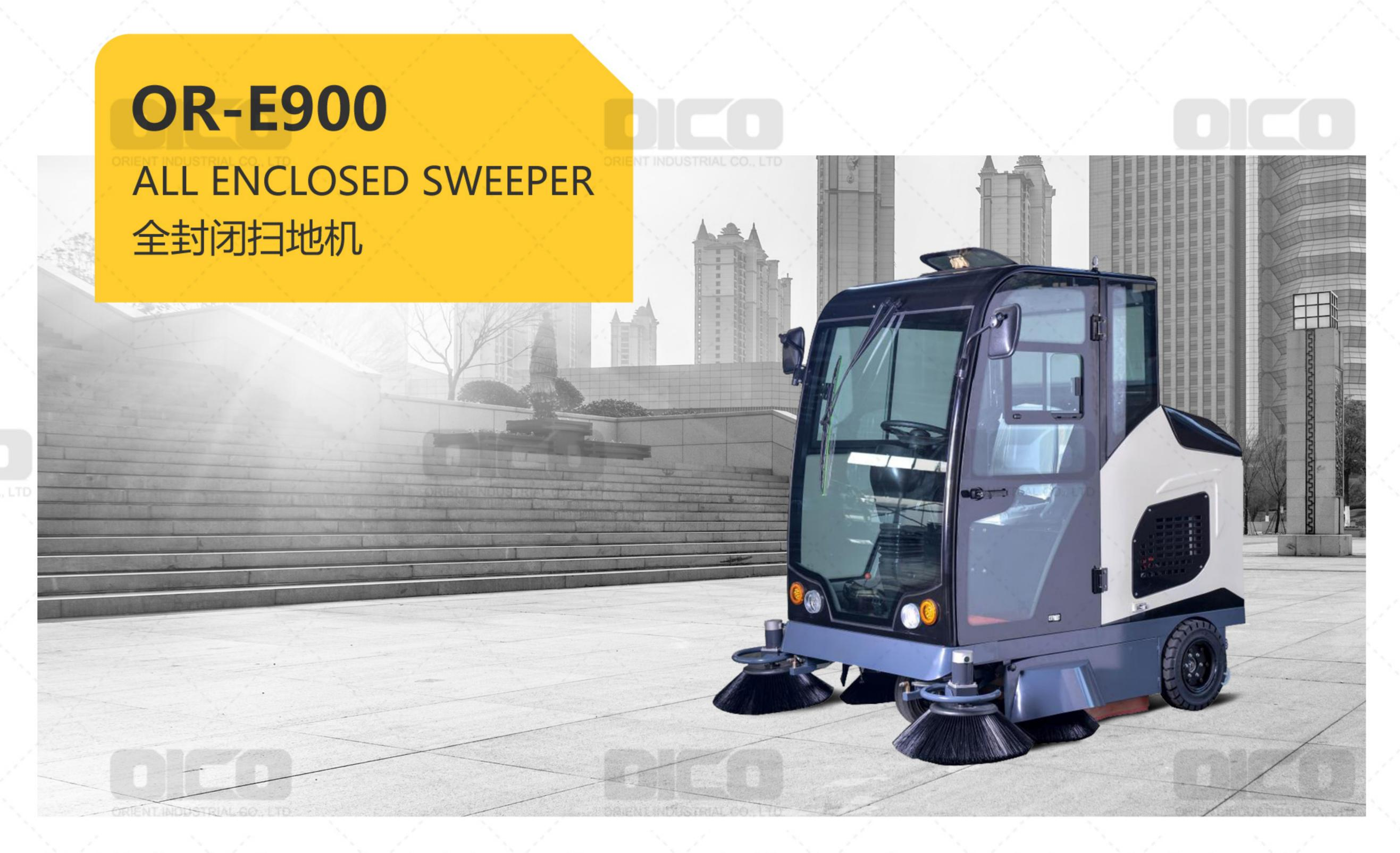
OR-E900 all enclosed sweeper has high cleaning efficiency. The double side brushes work at high speed make the working efficiency is up to 18000m²/h, which can easily solve various cleaning problems. It can clean up dust, stones, wood chips, glass and other garbage. It is suitable for operation on the flat ground such as cement, asphalt, ceramic tile, marble, etc., and can clean dust, stones, wood chips, glass and other garbage.
